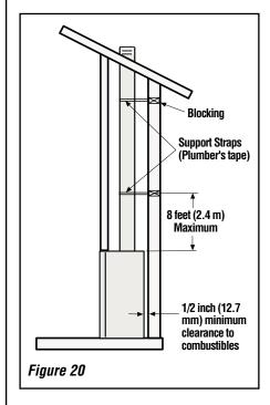
One method of support is by utilizing field provided support straps (conventional plumber's tape). Secure the plumber's tape to the framing members with nails or screws. Loop the tape around the vent, securing the ends of the tape to the framing. If desired, sheet metal screws #6 x 1/2" length may be used to secure the support straps to the vent pipe. Refer to *Figure 20*.
